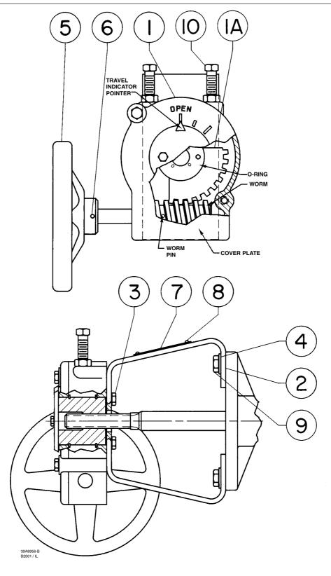
Figure 6. Type 1077 Actuator Assembly for Splined Shaft
